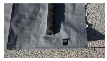
3. Loop the rear lacing line through the tie rod as shown in the picture. Start at the port side of the trampoline.
