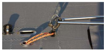
3. Feed the knot through the loop and pull.
