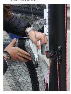
8. Insert the diagonal DS batten inside it's pocket and tension it as described in **5.5 Battens**.
