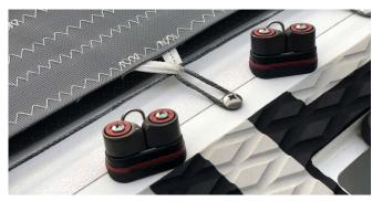
8. Attach the carbo 57mm ratchamatic single/swivel and the spring to the strap eye on both sides.
