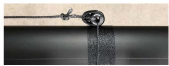
4. Install the block line to the top of the block and the strapeye above. Fixate the block on the same height as the bale line is positioned.
