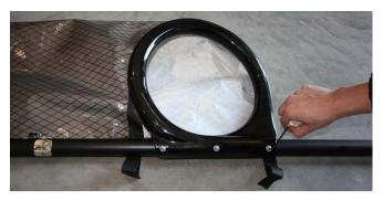
5. Install the snufferbag on the spipole using the velcro band.
