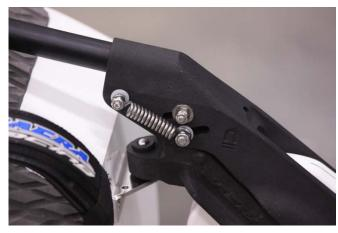
8. Take the philips screw out of the tillerarm.
