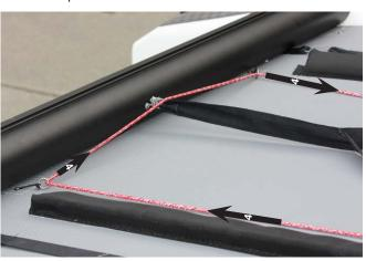
5. Feed the line through the 29mm block in front of the ovel grommet and pull the line underneath the trampoline.
