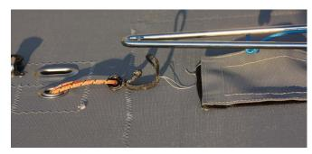
2. Feed the loop through to the mast rotator wishbone.
