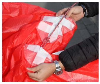
4. Divide the spin sheet in two egual lengths and loop the sheet through itself as shown in the picture.
