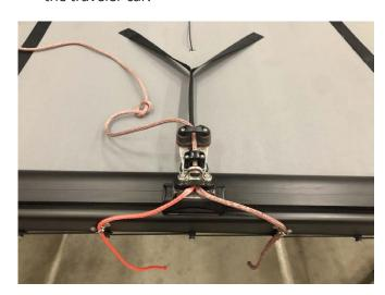
4. Knot the ends to the strapeyes. Make sure the traveler car is in the middle of the rear crossbar.
