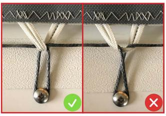
14. Tie the lacing line temporarily with half-hitch knot at the last loop.
