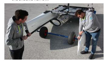
4. Knot the snufferline with a bowline around the pole and insert it in the slot of the ring.
