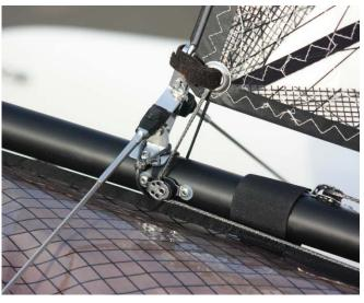
7. Attach the jibsheet small to the clew of the sail.
